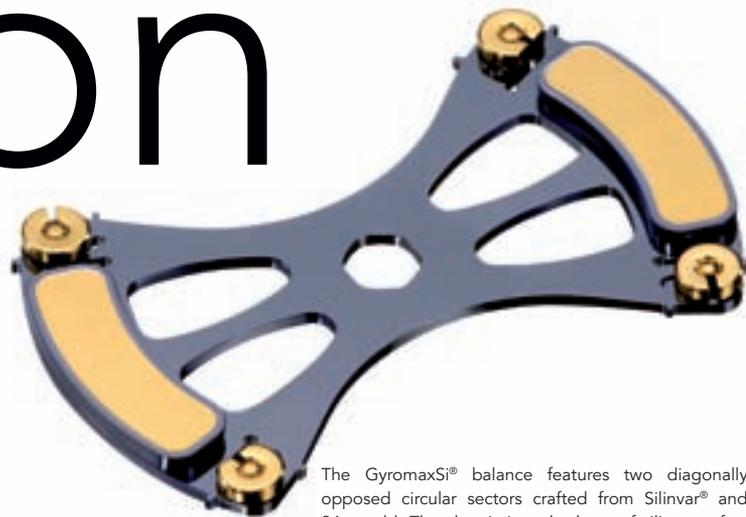
The GyromaxSi® balance features two diagonally opposed circular sectors crafted from Silinvar® and 24ct gold. The chassis is etched out of silicon wafers using the DRIE process and converted into a Silinvar® component by way of oxidation. The centrifugal masses are gold inlays integrated into the chassis with a technique patented by Patek Philippe. Additionally, the GyromaxSi® balance features four small slotted poising weights that can be precision-adjusted.
