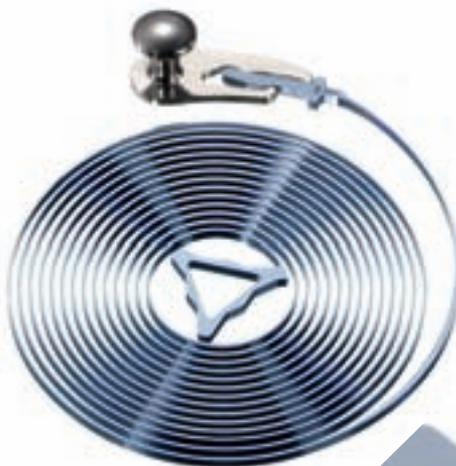
Thanks to the superior material properties of Silinvar® – which allows the balance spring to be three times flatter than a Breguet spring – the terminal curve and the integrated collet and stud attachment, the Spiromax® balance spring makes a decisive contribution to the isochronism of the movement. It is antimagnetic, corrosion-resistant, shock-resistant and insusceptible to temperature fluctuations.
