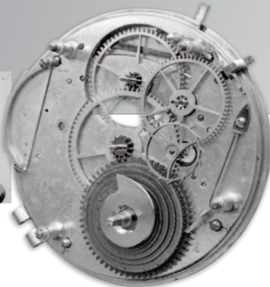
wheel (as yet uncompensated for temperature) with its flat spring.
