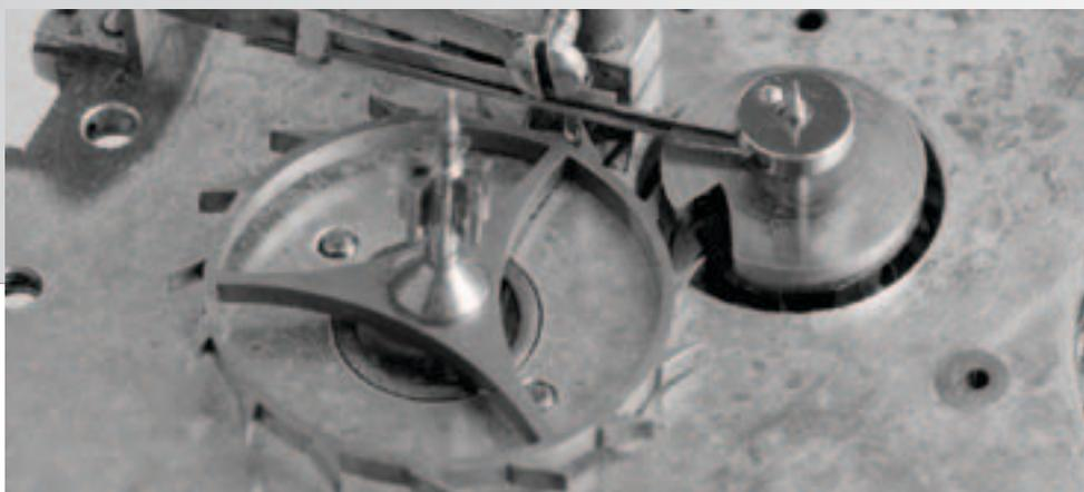
Left: Earnshaw's 'detached' spring detent chronometer escapement, underside of the movement's top plate from the "Jessop" pocket chronometer.
