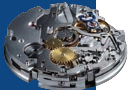
View of the 9907 MC movement, which reveals the chronograph mechanism and notably the flexible linear hammer, the chronograph's column wheel, the balance in gold-coloured Glucydur and its regulator in the form of the Cartier 'C'.
