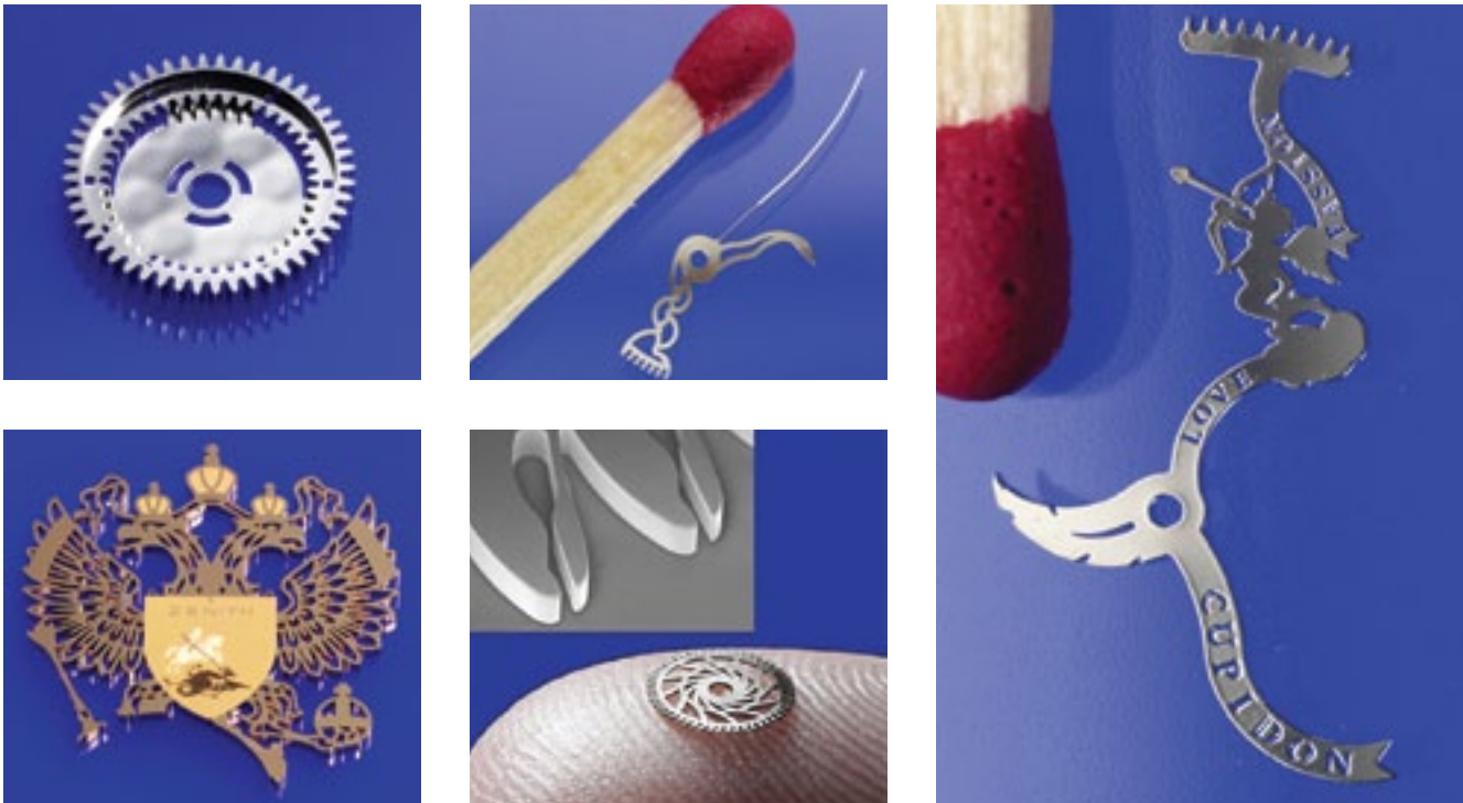
A selection of parts made by Mimotec using the UV LIGA technique.
