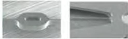
The heart of the G-P system is a complex frame etched in one-piece from a silicon wafer. The electron micrographs show detail of the areas arrowed. The hair-like strip across the centre forms the remontoir spring. The vertical element at the centre is part of the impulse lever. Other components (right) are one of the escape wheels, the winding lever and the remainder of the impulse lever.
