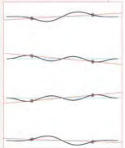
Energy states in the Girard Perregaux escapement remontoir spring. The red line shows the tilt of the winding arms. **A** and **D** are the low energy states after delivery of impulse. **B** and **C** are high energy 'meta stable' states produced by the gear train and the winding lever. The sequence of states is **A, B, C, D**, and back again.
