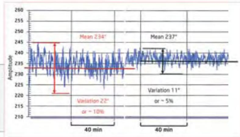
Variations in the energy delivered to the escapement by the standard gear train cause a pattern of variation in the amplitude of the balance. By closely examining these variations watchmakers can identify further imperfections in particular components in the gear train.
