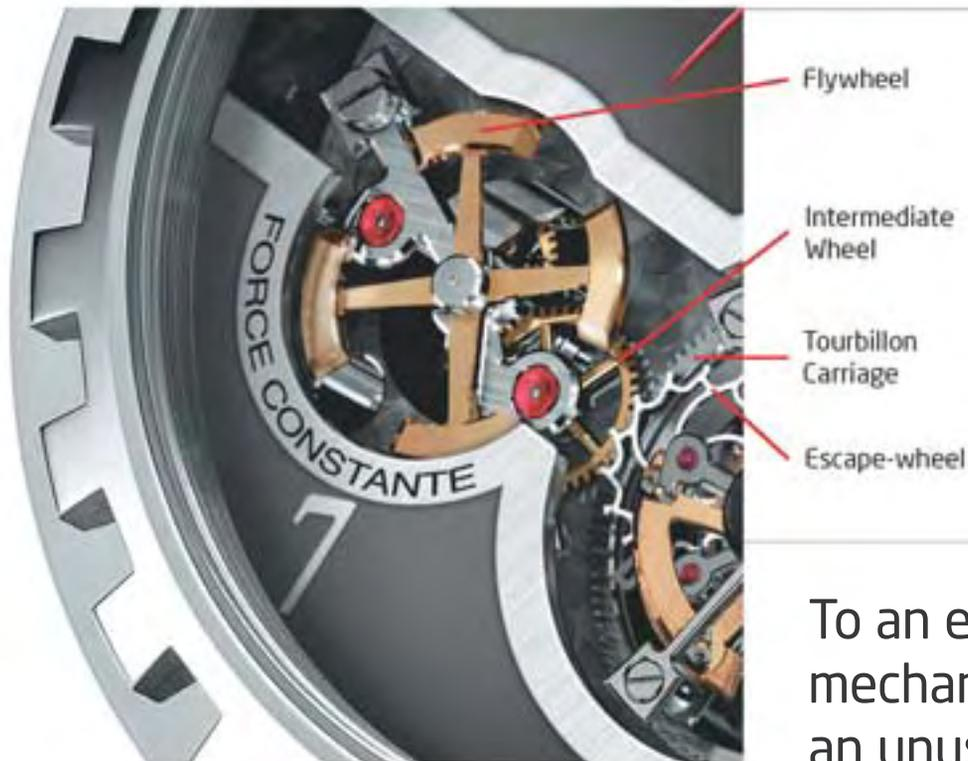
In the Academia Tourbillon the gear train applies torque to a 4-armed weight on the 4<sup>th</sup> wheel. This energy tensions a spiral spring attached to a sleeve on its arbor forming a reservoir of energy for transfer to an intermediate wheel that drives the tourbillon carriage providing a more constant and immediate source of impulse to the balance. Note the unusual shape of the escape wheel; it is made from nickel by electroforming.
