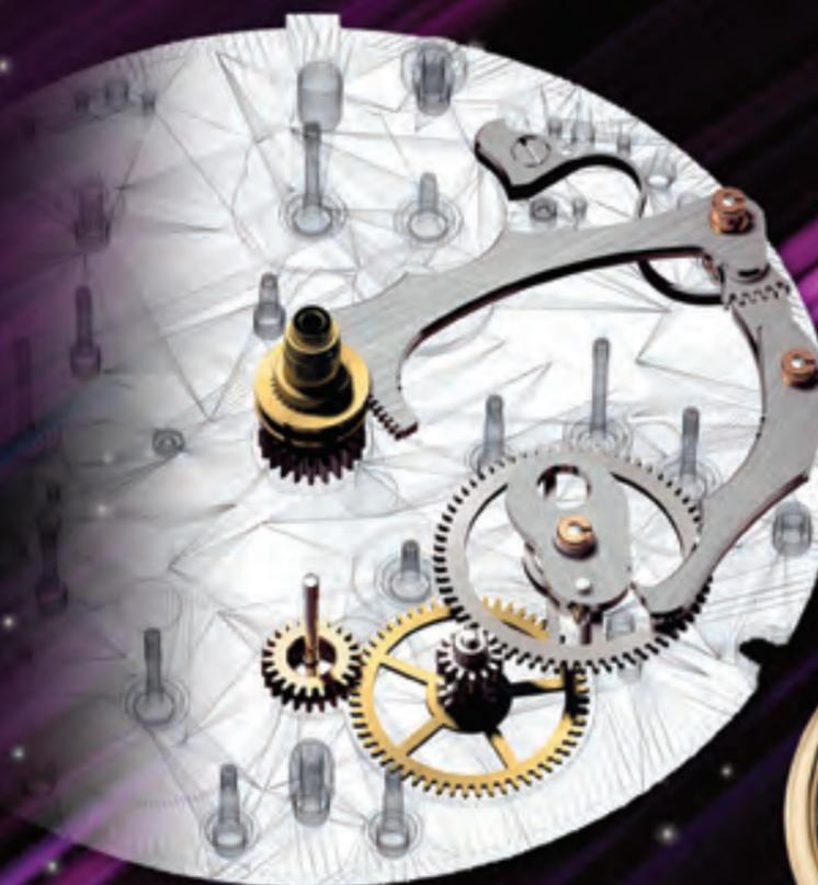
The Audemars Piguet Equation of Time mechanism. The wheel on which the equation cam is mounted is turned once a year by the calendar mechanism. The spring forces the lower end of the lever system to follow the cam. The teeth at the other end move the Equation hand from the dial centre.
