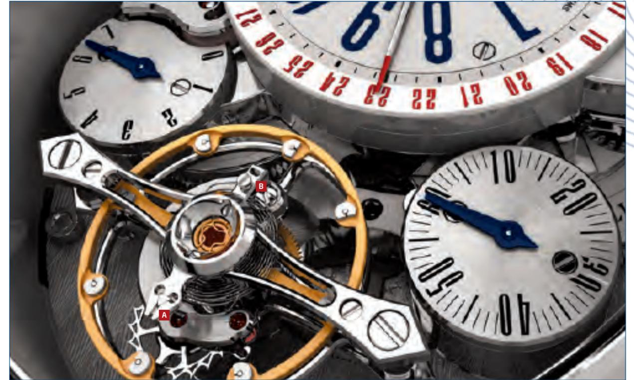
(Below) The Audemars Piguet Millenay Tourbillon in the 'Tradition of Excellence' series. With perpetual calendar, 7-day power reserve, dead-beat seconds and a completely new escapement, its double balance spring (above) went almost unnoticed. Note that the studs (A stud for upper balance spring and B stud for lower balance spring) to which the outer end of each spring is fixed are opposite sides of the balance centre and that each spring spirals in an anti-clockwise direction towards the centre.
