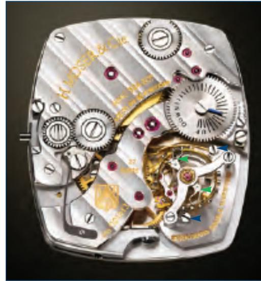
(Far left) Movement of the Henry watch. The unique Straumann double balance spring escapement module is positioned by the two screws (blue arrows) and can be exchanged for servicing if required greatly reducing the time for which the owner must relinquish his watch. The outer ends of each of the two balance springs are fixed to the studs (green arrows). The 4-day power reserve indicator is above right. The escape wheel is in hardened gold and does not require lubrication.
