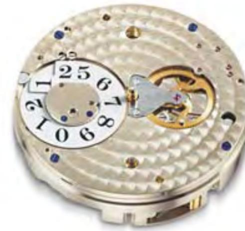
The under-dial view of the movement shows the large date display (indicating 25). The seconds arbor is at 6 o'clock and the power reserve mechanism towards 3. Note that the arbor for the minutes hand in the centre of the movement is not the centre arbor; this has been displaced by the large spring barrels. Extra gears are required to transfer the action of the centre arbor to the centre of the watch.
