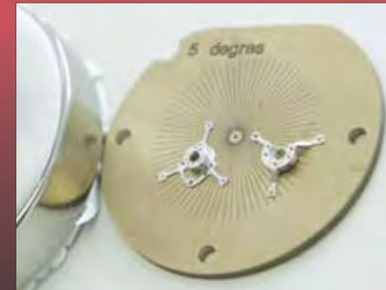
(Anticlockwise from top) Magnesium after 'decolletage', the milled magnesium alloy block, and the final tourbillon carriage before assembly. The alloy is two-and-a-half times lighter than titanium, and reduces energy loss due to friction and thus further improves the exceptional efficiency of the regulator.
