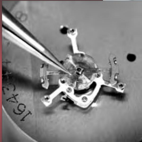
(Above) The H-shaped balance is made from platinum iridium, one of the densest materials known. The shape is optimised aerodynamically (less 'skin friction') and the inertia:mass ratio, aided by openworked arms, makes it a better oscillator. Note the gold timing screws; this is a 'free-sprung' balance.
