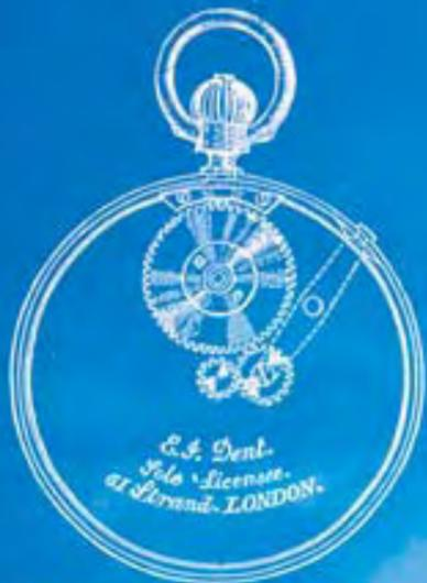
The First Watch Winding and Setting the Hands without a Key. Patented and Introduced by E. I. DENT. (Trade Mark
