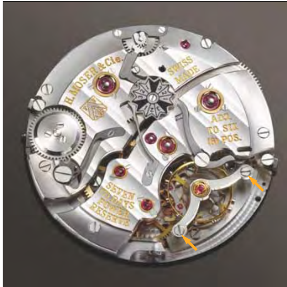
(Left) Rear view of the Perpetual 1's HMC341 movement. The leap-year indicator turns once in 12 years. If the watch has been stopped for some time, the pusher at the side of the case sets the year by operating on the L-shaped lever pivoted above the balance. In leap years a cam under the leap year indicator will, via the L-shaped lever pivoted above the indicator, feed back to the date mechanism to give a 29-day month. Uniquely to Moser, the balance and escapement assembly can be removed simply by undoing two screws (marked). (Below) The Perpetual 1's double-pull crown mechanism, shown in the outer-most 'hand-set' position. In 'date-adjust' the curved piece (arrow) is rotated so that the wheel attached to it comes into mesh with 'D', which turns the date rings. Uniquely, date adjustment can be made in either direction at any time of day. The curved piece engages via a slotted arm and a click system that, again uniquely, unambiguously selects the crown positions. The crown is pulled into date-set and then released before pulling again to get into 'hand-set'. Thus, the tiresome search for the central 'date-adjust' crown position is now a thing of the past.
