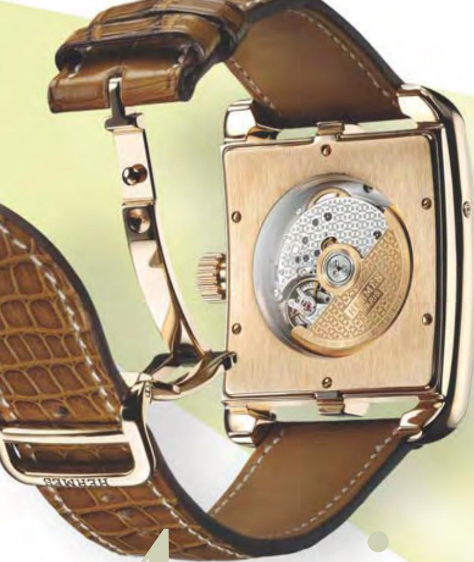
Hermès' big launch for Baselworld 2007 is this astronomic watch (£18,150) - the second of the Parisian house's 'Cape Cod' models to receive a Vaucher Manufacture Fleurier movement. Here, calibre H 1929 drives hours, minutes, seconds, retrograde date and moon phases, which are accurate for 122 years and 46 days (after which, a one-day correction is required). Issued in respective series of 170 rose- and white-gold pieces; a number corresponding to the years since Hermès' foundation in 1837.
