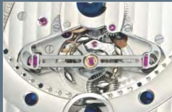
(Above) With its movement reversed, De Bethune’s DB S displays its titanium triple-shock-protection balance. The four torpedo-shaped platinum weights of the balance can be seen under the bridge.
