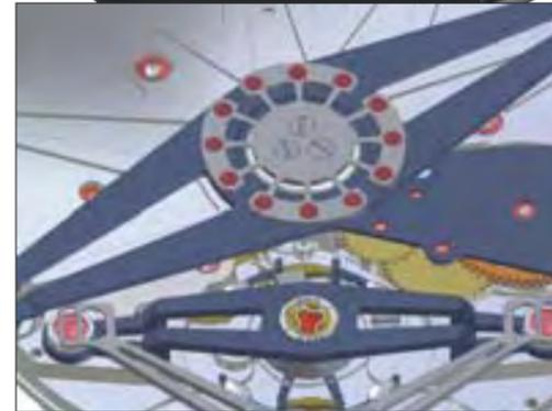
(Above) De Bethune's experience with titanium has enabled the use of the lightweight but strong metal in both the balance bridge and the rotor arms of the new automatic movement in the Power. As a result, the rotor (like the balance) has the highest inertia:mass ratio available today.
