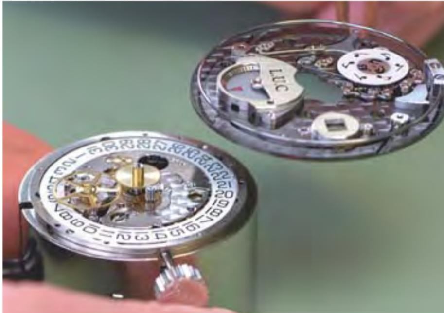
and a resulting stability of rate. The twin spring barrels were able to hold 65-70 hours running time, half as much again as was usual at the time, and a feature that has been much copied since.
