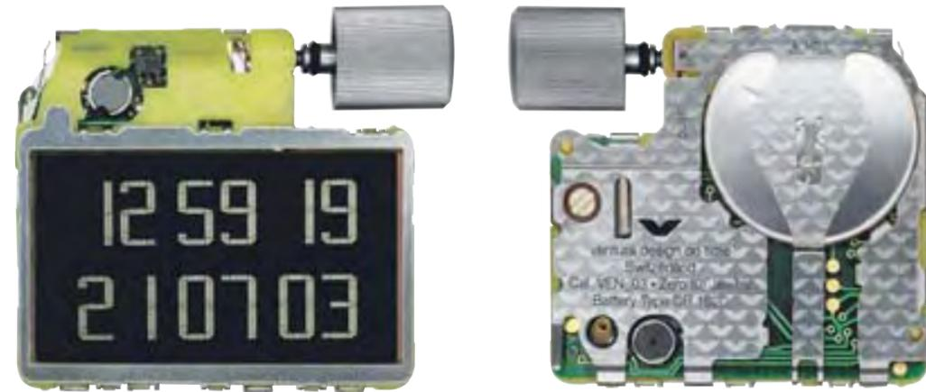
(Left) Front and rear views of the battery-powered VEN\_04 calibre made by Ventura and used for the v-tec Sigma and v-tec Delta models. Its functions are operated by the EasySkroll system, using the fluted crown protruding from the top.
