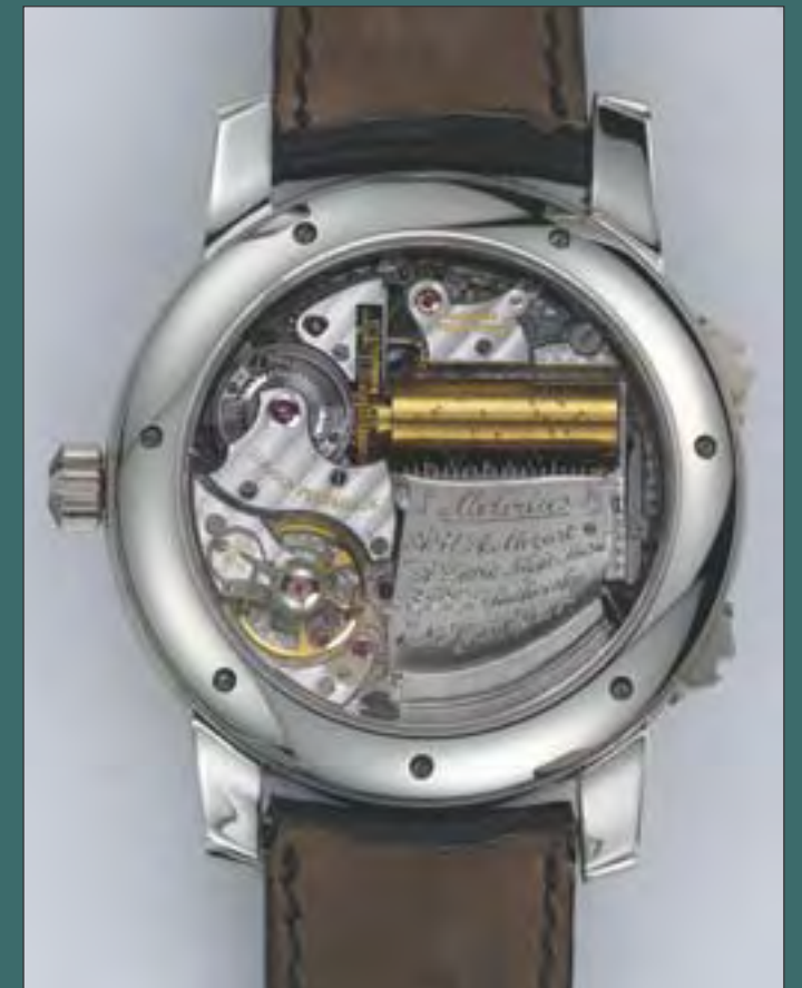
(Above-right and right) Girard-Perregaux's Opera Three (SFr.545,000) uses a mechanism developed originally by Claret for an unsuccessful self-branded watch. The movement is composed of a miniature keyboard with 20 tonal 'tines' or blades strummed by a drum furnished with some 150 pins. A selector makes it possible to choose between two different melodies, by shifting the drum sideways. The melodies can be personalised on request - within the given 20 notes of course!
