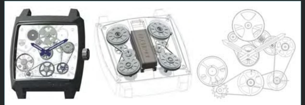
(Above) The intended arrangement for the V4's rubber belts, which replace wheels at several stages throughout the going train.
