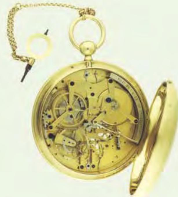
(Above) Journe's sixth pocket watch uses a fusée and chain to equalise the torque fed into the gear train by the mainspring as it unwinds. A chain of tiny, handmade links (just visible here, round the circumference of the barrel) uncoils from a stepped cone, graduating the leverage. Dr Gschwind's commission also houses a five-second remontoir and a detent escapement.
