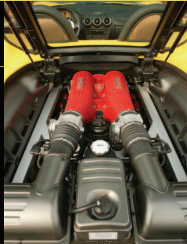
(Left) The F430 Spider's 90° V8 engine, at the rear of the car (only the 12-cylinder Ferraris have the engine at the front). The Spider's finely tuned aerodynamics ensure optimal comfort for the driver in terms of wind and noise when the roof is down.
