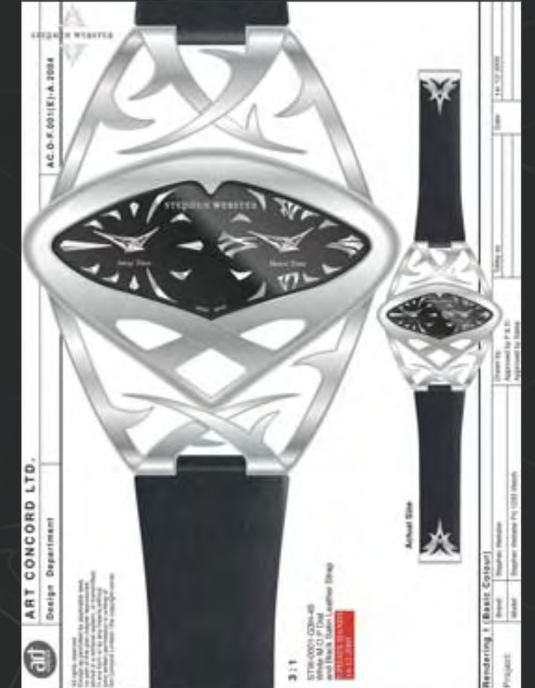
(Right) Design diagrams from the Libertine's final development stages. The 'Away Time' and 'Home Time' dial text was eventually removed, and '3, 6, 9, 12' indexes were added to the away-time subdial.
