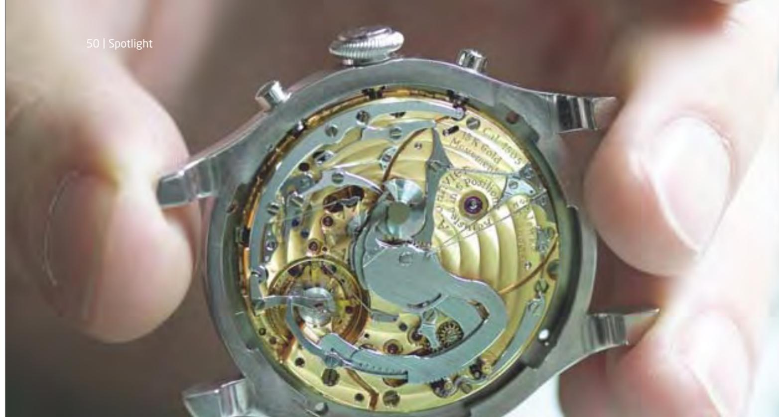
(Above) The construction of the movement, with the hours and minutes off-centre, allows the striking-racks to be mounted in the centre of the movement. This in turn makes oversized racks possible, for greater precision and control. The visible Anachron balance spring oscillates at a frequency of 21,600 vph.
