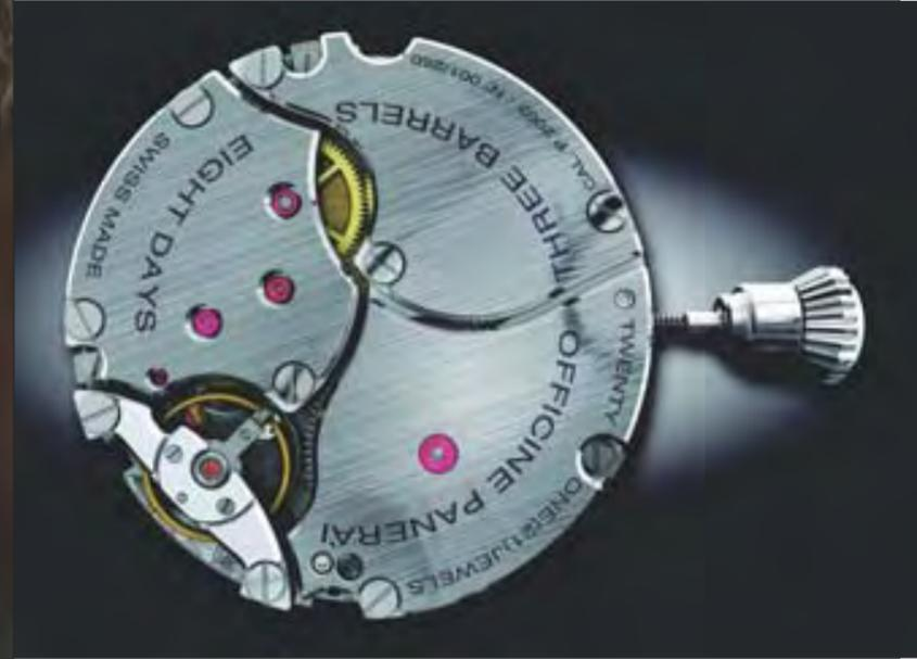
Fresh out of Neuchâtel, the new calibre P.2002 - a manual-wind, 21-jewel, 245-part, 28,800 vph, triple-barrel movement with eight-day power reserve - a nod to the 8-day Angelus movements used by Panerai since the 1940s.
