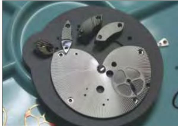
(Above) The five spindle-shaped bridges, which give the Fuseau de l'infini collection (of which the Luvoréne 1 is a part) its name.
