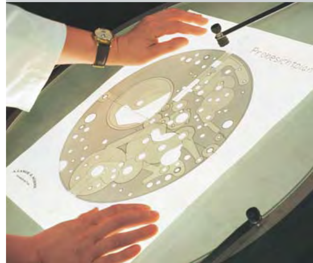
(Below) Visual inspection of a Lange baseplate with a projector. A light-projected enlargement is compared to a transparent engineering drawing at the same scale.
