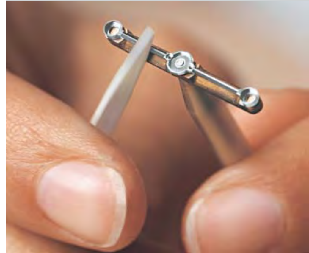
(Above) Final polishing of the tourbillon bridge.
