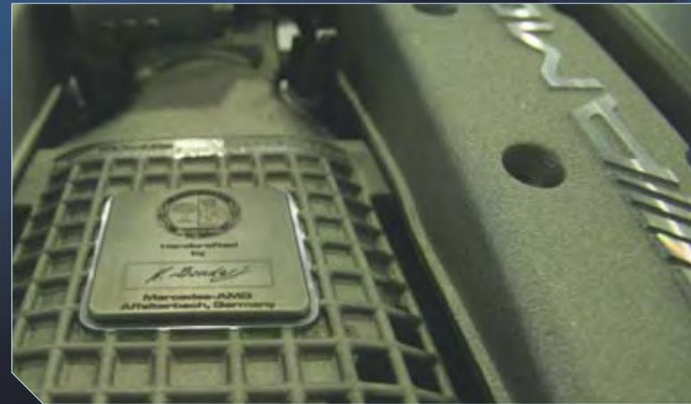
The signature plate on all completed AMG engines is a source of great pride to the engineer involved, and reinforces the 'one man, one engine' ethos.
