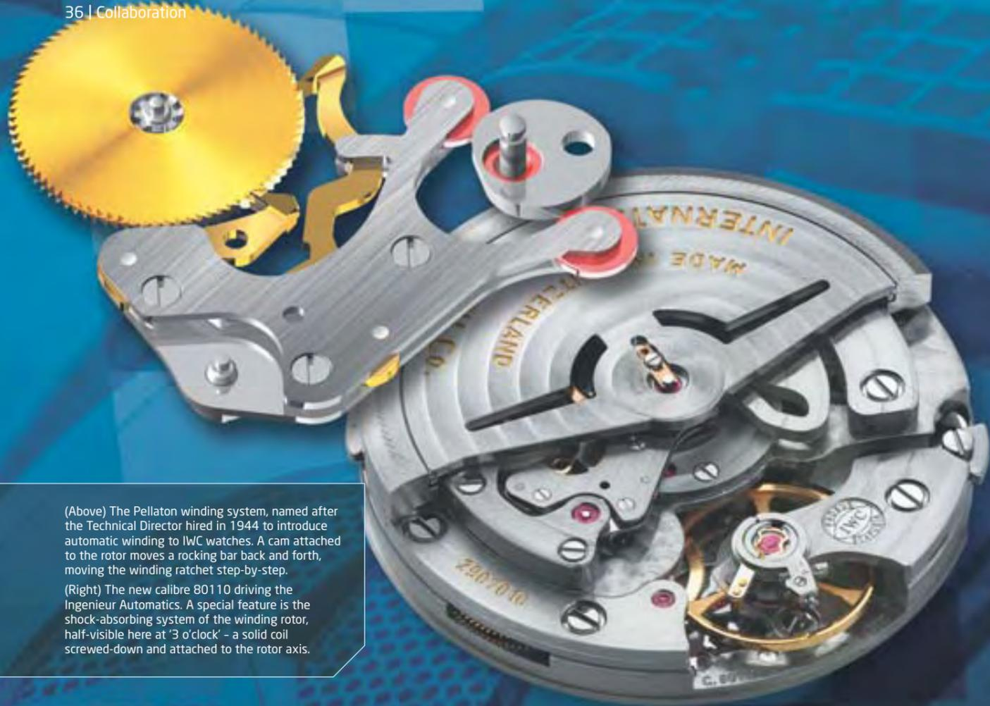
(Above) The Pellaton winding system, named after the Technical Director hired in 1944 to introduce automatic winding to IWC watches. A cam attached to the rotor moves a rocking bar back and forth, moving the winding ratchet step-by-step.
