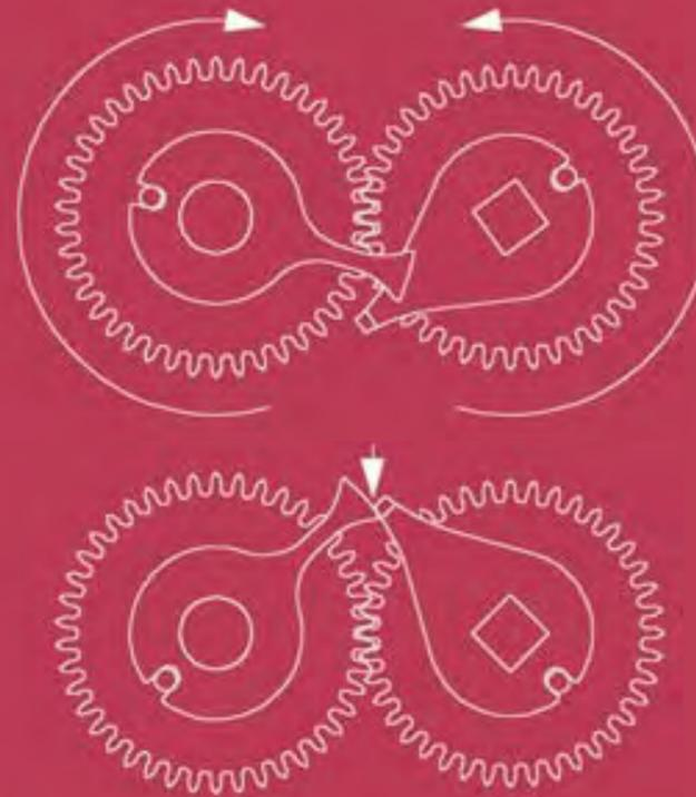
Detail diagram of the over-winding limiting system. (Top) As the two barrels are wound, the 'fingers' pass over each other. (Bottom) Here, a maximum state of wind has been reached in both barrels, and the two fingers have finally coincided after 20.75 turns, jamming any further winding.
