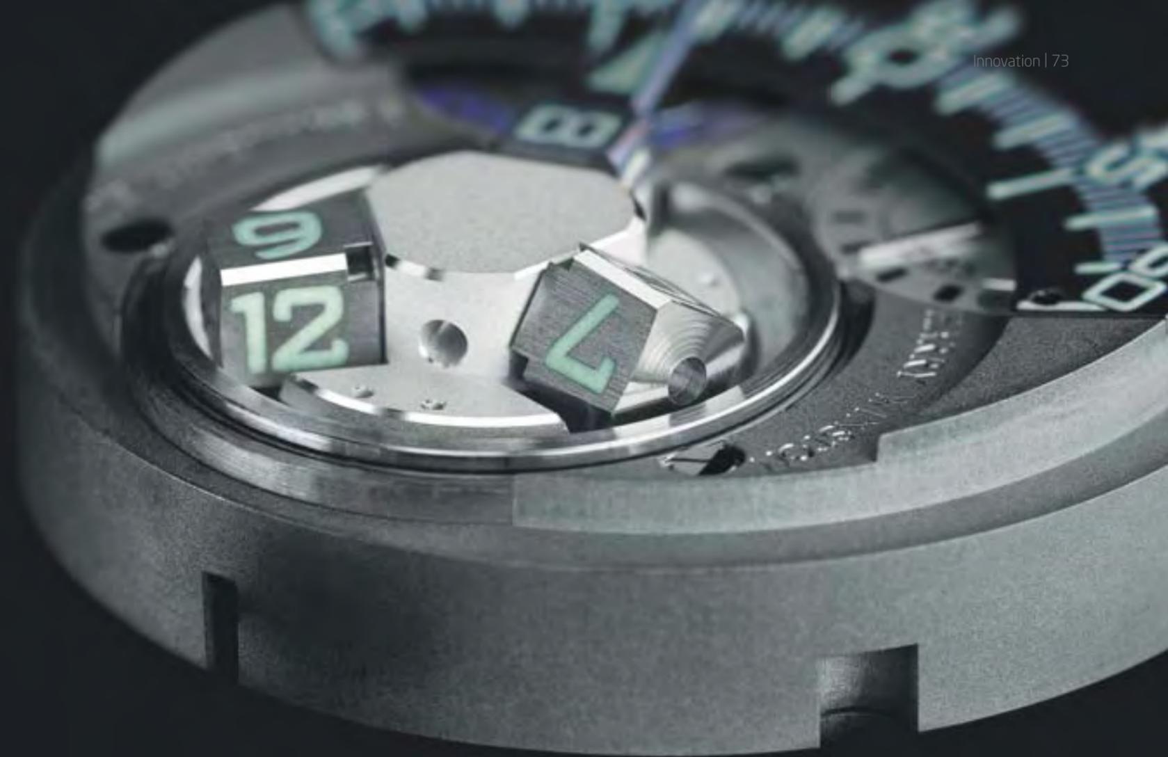
Since the minute hand has to cover a long distance (120°) before returning to zero, it is brought back by a highly resistant traction spring, wound by a ring fixed to the ball-bearing mechanism. The satellite-hour system, as it turns, drives the entire ring. When the hand reaches the figure 60, a double star is released, in turn releasing the spring.
