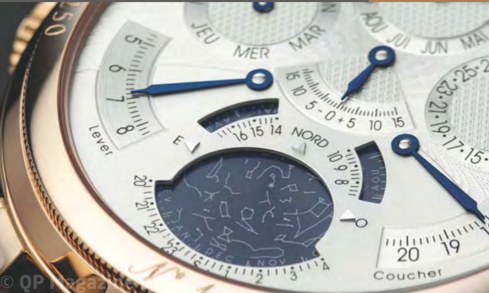
Detail of the Tour de l'Île's rear display. The Northern Hemisphere star chart is capped by the dials of the perpetual calendar arranged in a triangle, a blued hand in the centre shows the equation of time (the running difference between solar time and mean time) and two segments at 4 o'clock and 8 o'clock give sunrise and sunset times.
