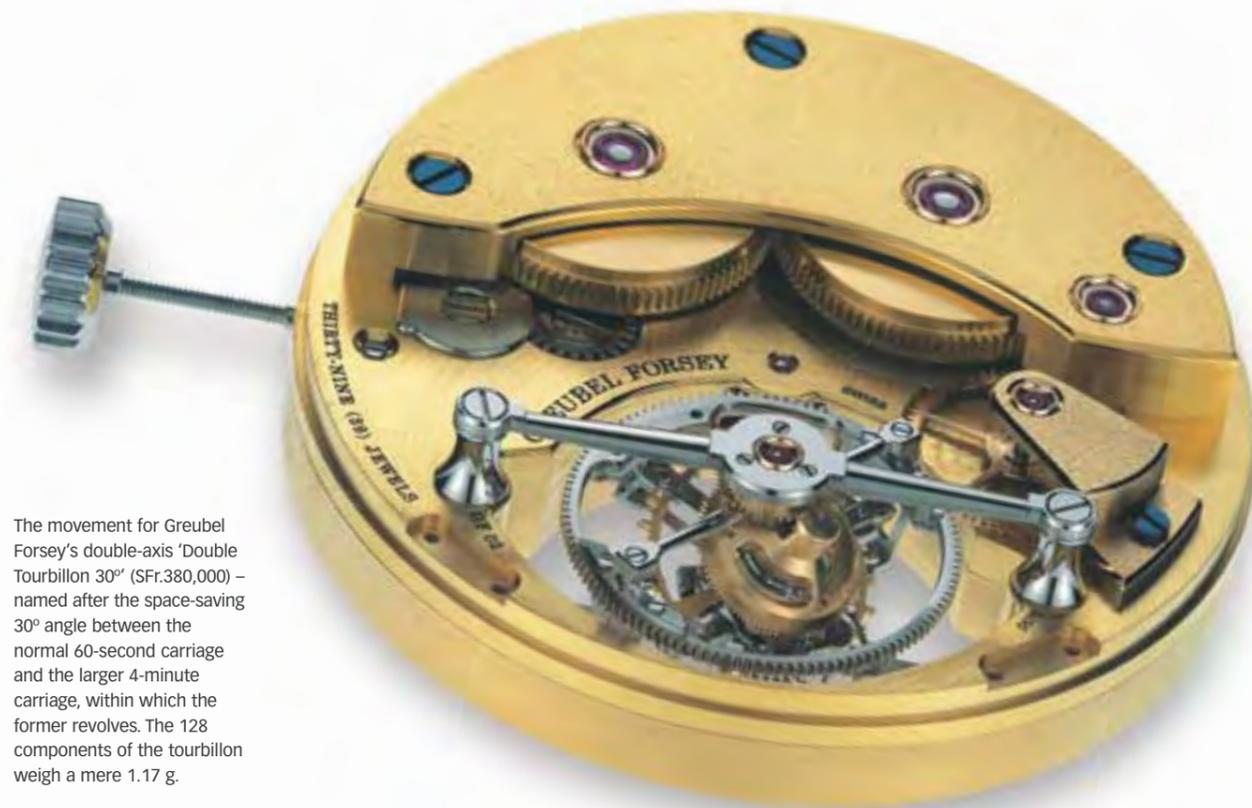
The movement for Greubel Forsey's double-axis 'Double Tourbillon 30°' (SFr.380,000) – named after the space-saving 30° angle between the normal 60-second carriage and the larger 4-minute carriage, within which the former revolves. The 128 components of the tourbillon weigh a mere 1.17 g.
