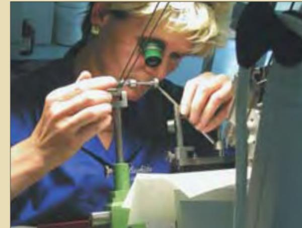
(Left) Great care is taken in polishing the angles of the steel components. The part being polished is mounted on special holder and the edges are pressed firmly against a rapidly rotating tungsten carbide lap.
