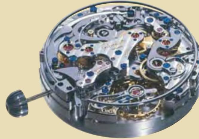
(Above) The movement of the PanoRetroGraph shows the features of a top Glashütte Original watch. The steel work has a flat, grained finish achieved on a tin block in the traditional way. Edges are angled and crisp, the screws are blue, and the jewels are set in gold chatons. This permits very precise adjustment of the gears' meshing during assembly, giving a very smooth delivery of power to the escapement. The raised peripheral ring is the gong, struck at the end of countdown timing.
