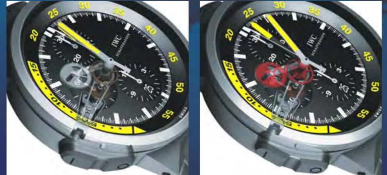
These two diagrams show the world premiere 'Minute Memory' function, found exclusively in the eponymous Aquatimer model. (Left) In the 'off' position, the Minute Memory hand runs under the minute hand. (Right) In the 'on' position, the Minute Memory hand stops and the time is recorded.
