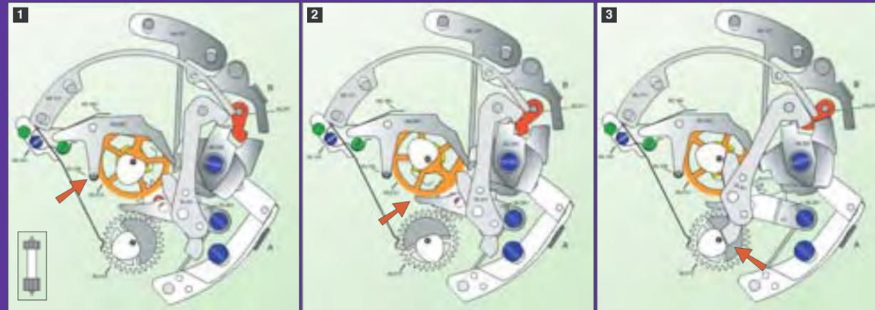
Operation of the 7750, viewed from the back of the movement with 12 o'clock at the bottom.
