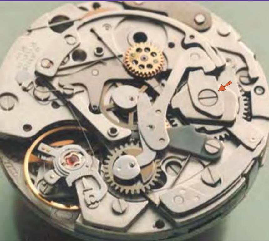
(Above) The basic Valjoux 7750 chronograph movement, shown with the winding module removed. The cams (arrow) interact with stubby levers to control the chronograph functions. These parts can be simply stamped out from sheet metal.
