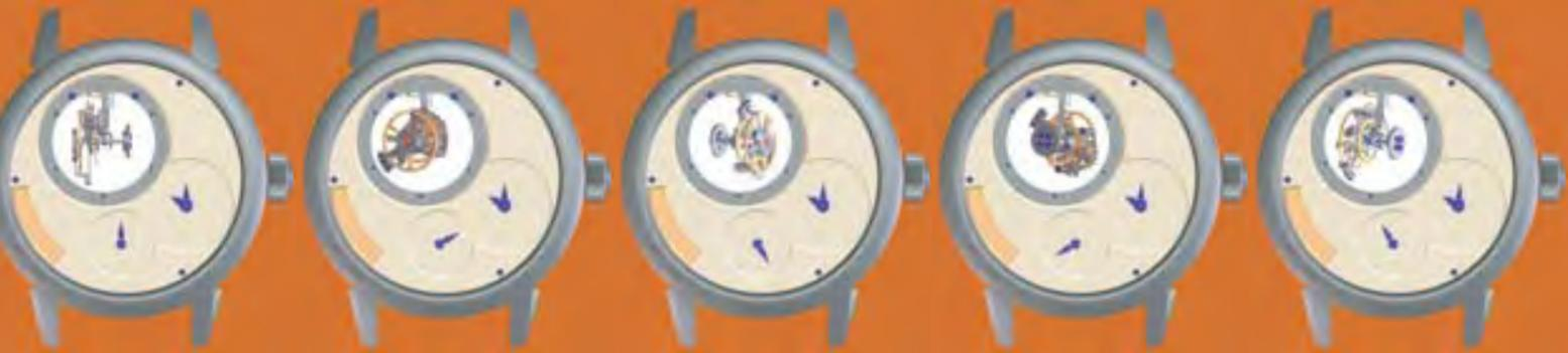
Sequence of diagrams charting the minute-long revolution of the tourbillon cage about the second axis.
