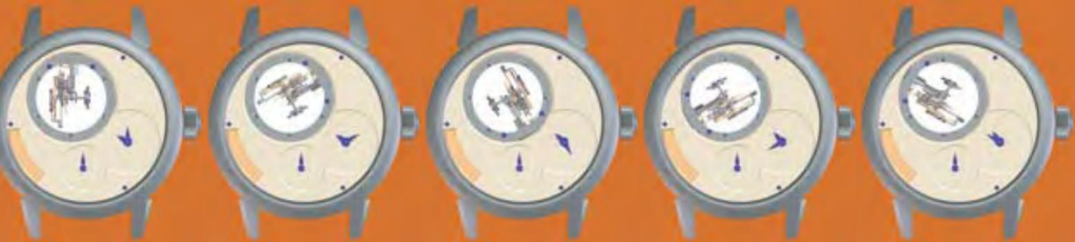
Sequence of diagrams charting the hour-long revolution of the tourbillon cage about the third axis.
