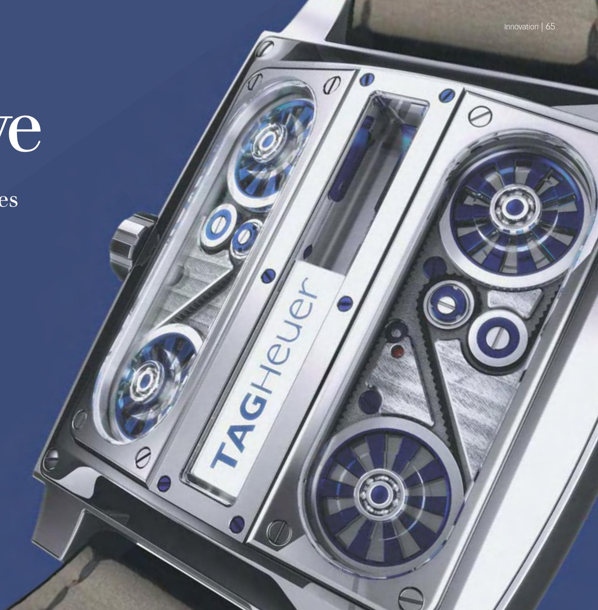
Two views of the Monaco V4 from the back and front (left and right respectively). The sapphire glass caseback allows an unobstructed view of the central linear oscillating winding weight and the four winding barrels, which are mounted on a V-shaped main plate angled at 15° like cylinders in a racing engine.
