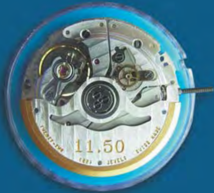
(Left) On the left side, some of the exchanger's gears for the rotor's unidirectional winding mechanism are clearly visible, with the balance wheel, balance spring, mobile stud holder, adjuster and Incabloc protection clearly visible on the right. (Right) The back view of the 11.50 STT movement, with the ball bearings just visible as specks of light in the circular section around the rotor's axis.
