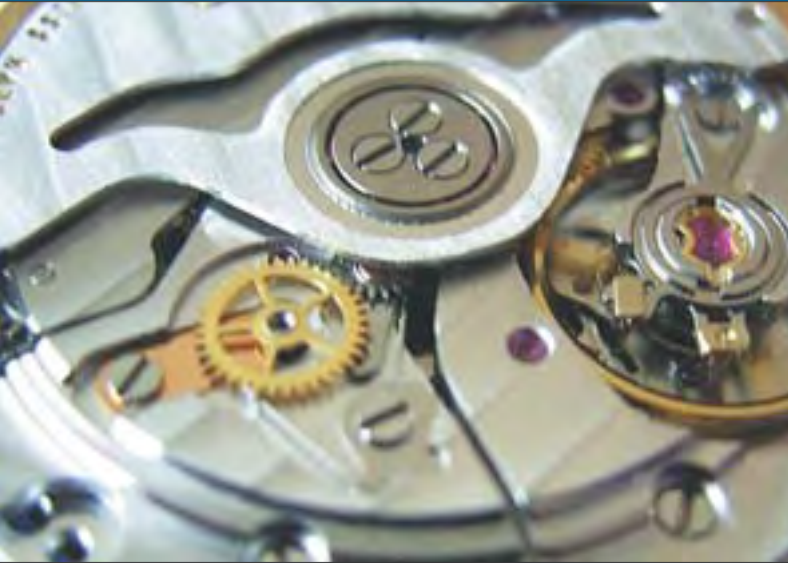
(Left) On the left side, some of the exchanger's gears for the rotor's unidirectional winding mechanism are clearly visible, with the balance wheel, balance spring, mobile stud holder, adjuster and Incabloc protection clearly visible on the right. (Right) The back view of the 11.50 STT movement, with the ball bearings just visible as specks of light in the circular section around the rotor's axis.
