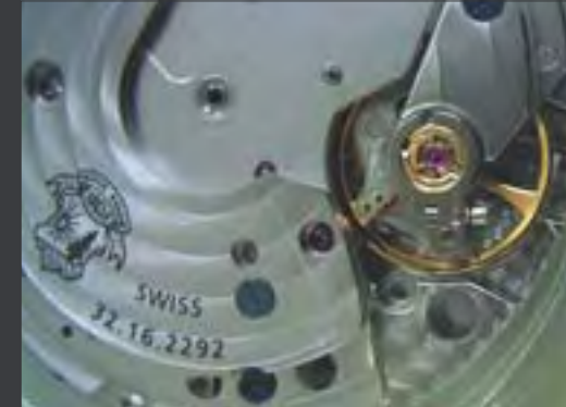
Back view of the movement. Note the depth of the movement and the circular-shaped Geneva stripes. The Ulysse Nardin logo, displayed on their first in-house movement manufactured in La Chaux-de-Fonds, is proudly visible.
