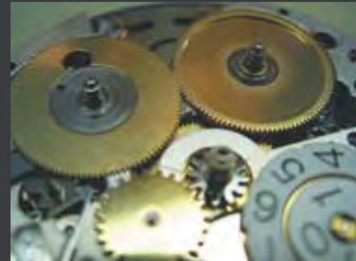
The upper layer of the movement (just below the dial), showing the countdown timer (left) and the alarm (right).
