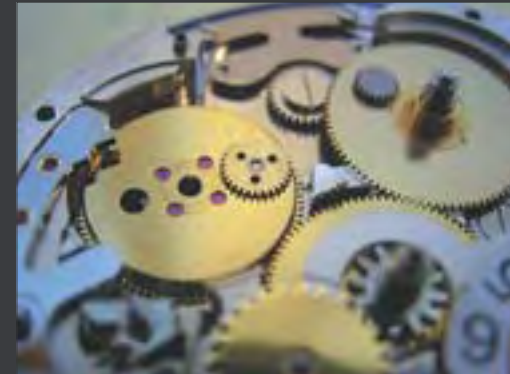
The second layer of the movement, exposing the pushers and a microscopic satellite wheel (almost spot centre in this picture) that is the key component of the differential's 'backwards and forwards' functionality.
