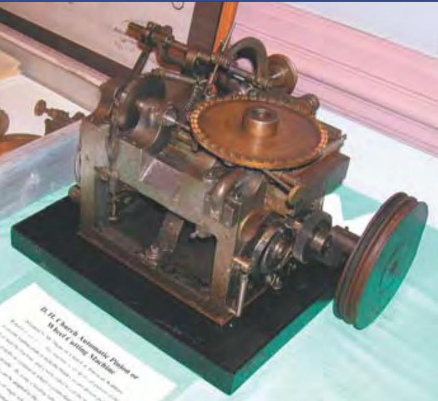
Automatic pinion cutting machine used by the Waltham Watch Company in 1892. The curved arm would automatically pierce a piece of metal from the carousel and the machine turned it into a watch pinion. All the operator had to do was to fill the carousel.
