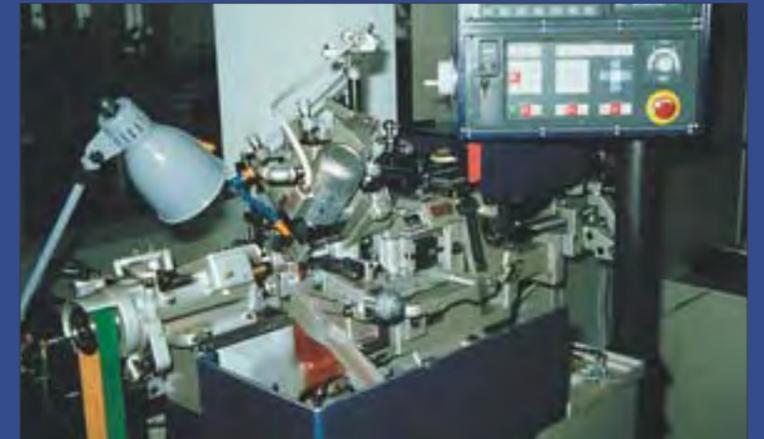
Modern Tornos lathe at Jaeger-LeCoultre. Tools are moved by stepping motors controlled by computer programs.
