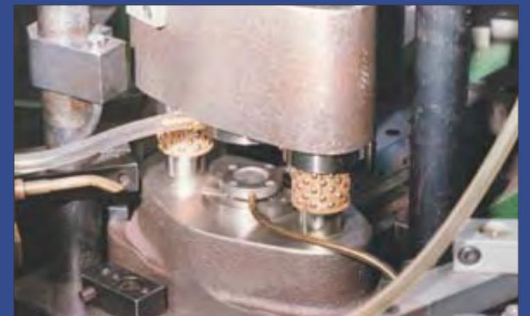
Modern Press Tool at Nivarox FAR, forming the lever for the Omega Coaxial Escapement.
