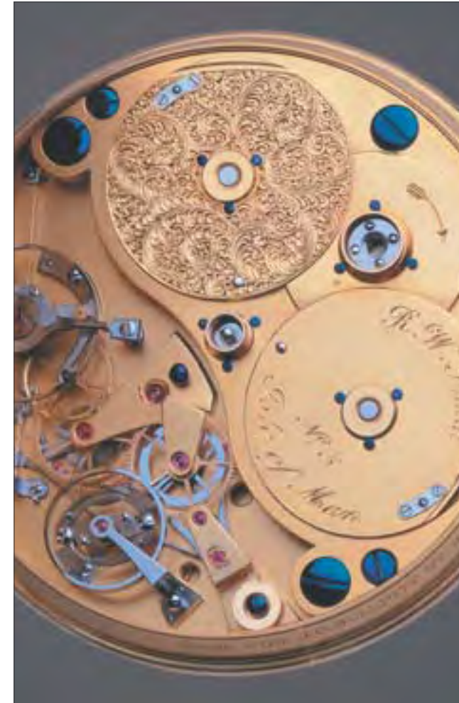
This, the Number 3 movement from RW Smith, demonstrates vastly different techniques to that of the Chopard calibre 1.96. The finish is known as 'frosting', or 'matting', and is applied to the surface by a spinning brass or steel mop. The surface is then gold plated, which prevents tarnishing. Also, note the screw heads, which have been anodised to impart a striking blue hue.
