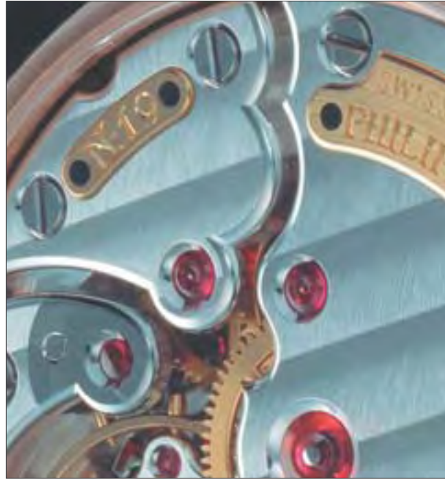
These two pictures show details from a Philippe Dufour wristwatch, perfectly exemplifying how handmade classical anglage should appear. A movement treated like this is the very picture of horological elegance.
