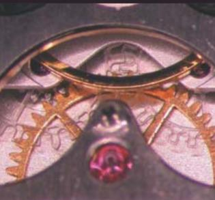
(Above) Functioning diamond balance spring mounted in the escapement. One arm of the balance wheel below is just visible near 6 o'clock. Although diamond is unbelievably tough and flexible insertion and regulation of the spring requires special techniques to avoid breakage. The balance spring stud, which holds the outer end of the balance spring is visible at 3 o'clock.
