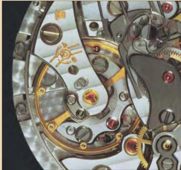
In the "free-sprung" Giromax balance by Patek Philippe, C-shaped weights placed around the balance wheel are used to adjust the rate. As indicated on the balance cock, turning the slot to face inwards (increasing the moment of inertia of the wheel) will cause the watch to go slower. Note that equal adjustments must be made to weights on opposite sides of the wheel to avoid altering the poise.
