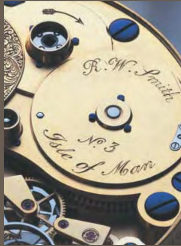
Word of the Number 2 Smith pocket watch quickly spread among collectors, and soon he was commissioned by a British client to make Number 3, an English-finished, twin-barrelled pocket watch with Peto cross detent escapement, state-of-wind indicator and the added complication of a 15-second remontoire, an extra spring mechanism that ensures a high degree of accuracy regardless of whether or not the watch is fully or only partly wound. It was to take around 4,000 hours to complete.
