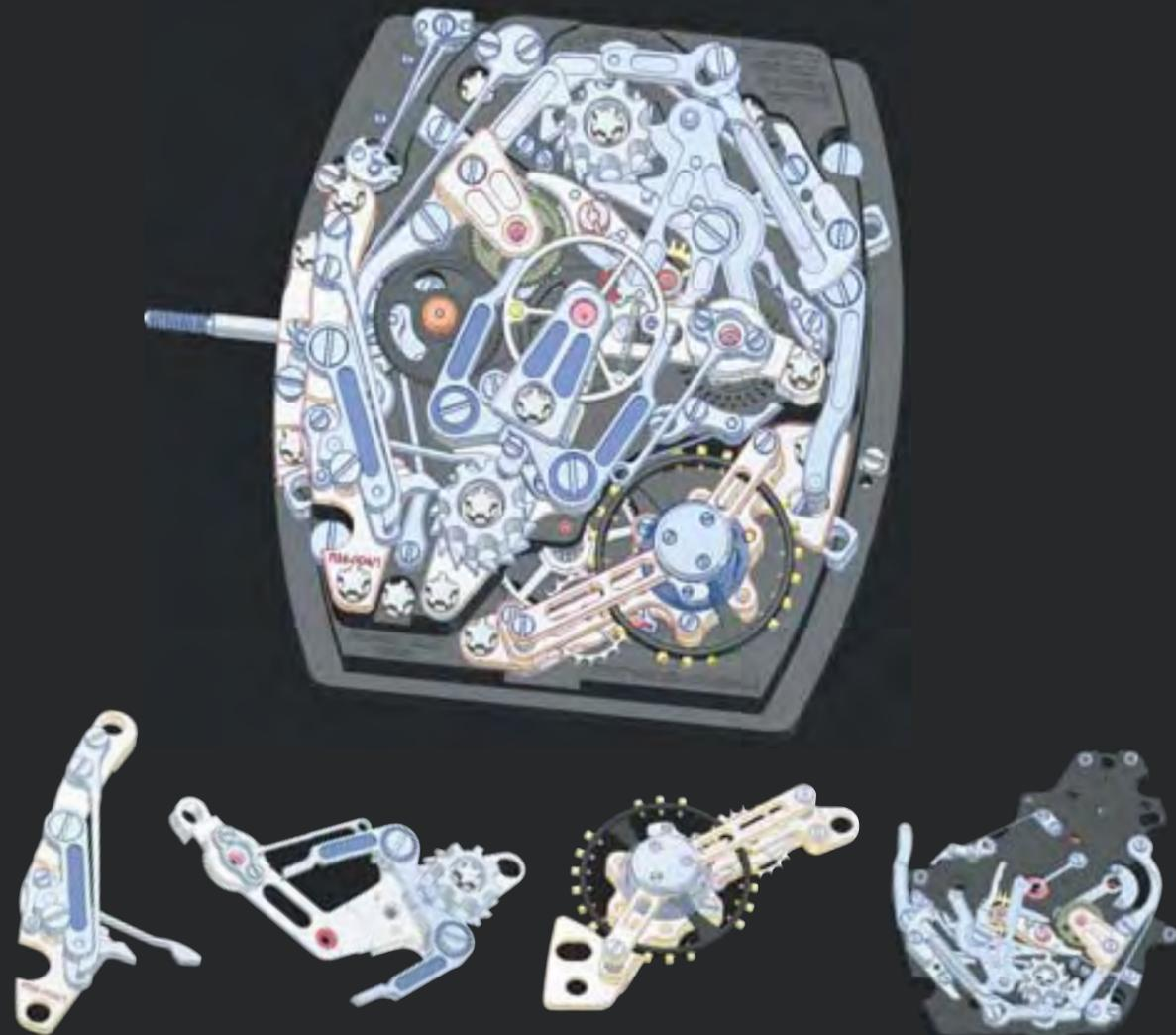
An example of the modular construction system, this picture shows the independent group of pushers and springs controlling the starting and stopping action of the chronograph's split seconds unit.
