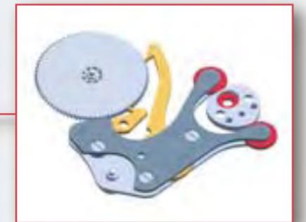
ment of the rotor. Allied to this is a large spring barrel capable of holding up to 200 hours' running time, and a device to stop the escapement after 186 hours (intended to prevent inaccurate running as the spring winds down). The movement has also been fitted with various refinements such as a Breguet balance spring.
