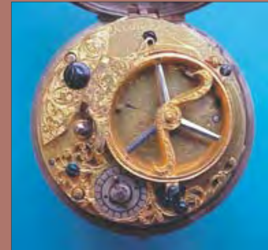
(Far left) The museum contains some historical pieces, including this Abraham-Louis Breguet self-winding watch, thought to be the earliest-surviving example.
