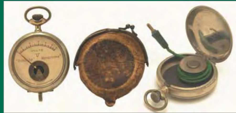
A pocket watch-style volt-meter, complete with leather case and wire, “for testing accumulators”.
