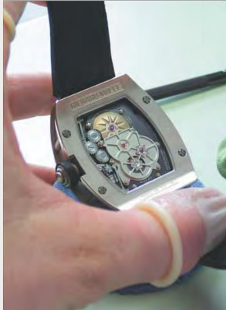
The reverse of the RM003 tourbillon. The Formula 1-inspired engineering behind Richard Mille's concept of watchmaking has led to the inclusion of a torque gauge to go alongside the power reserve. Above and beyond this though, the movement is constructed to withstand hard wear and tear – Richard Mille's party trick is to throw the watch to the floor!
