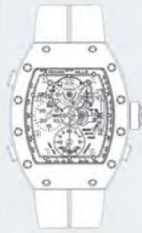
The chronograph movement for the RM004 is replete with innovations, ranging from improved split-second function to a new fast-winding spring barrel. There is even an improved escapement.
