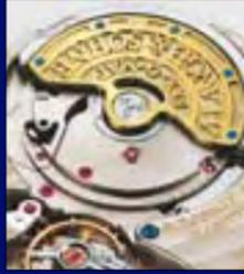
Automatic watches rely on the kinetic energy created by rotating weights to keep the watch wound. These usually occupy the whole diameter of the movement, but some companies use micro-rotors to allow their movements to be appreciated without obstruction.
