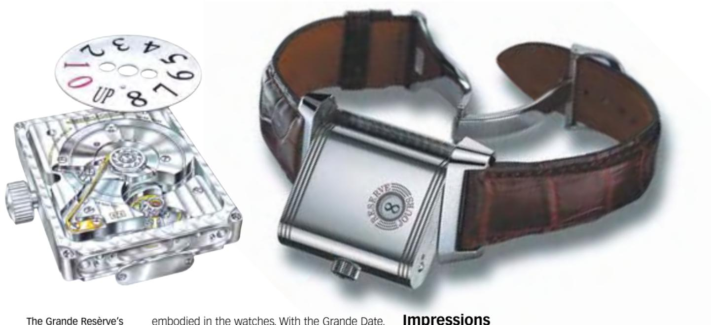
The Grande Réserve's whimsical method of displaying the remaining running time relies, nevertheless, on a complicated setup below the case back. The diagram shows the arrangement of clicks and wheels required to ensure that the disc jumps into place as the power reserve declines or increases with winding. There is also a mechanism to prevent the disc going beyond eight when winding.
